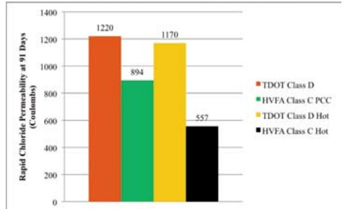
Figure 11: 91-day Rapid Chloride permeability of HVFA and TDOT Class D Mixtures
