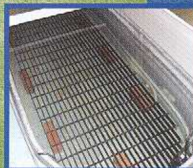
Figure 4. Grate supported by bricks
