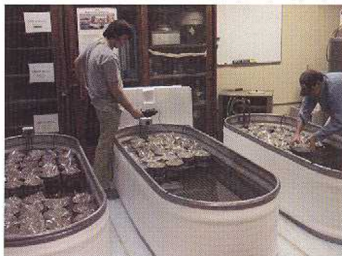
Figure 1. Activation of Maturity and Temperature Loggers
