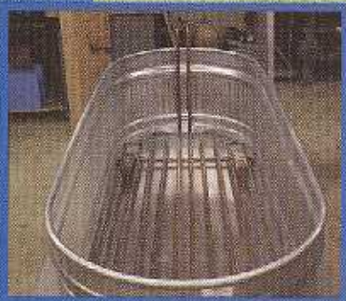
Figure 6. Copper Circulation Tubing
