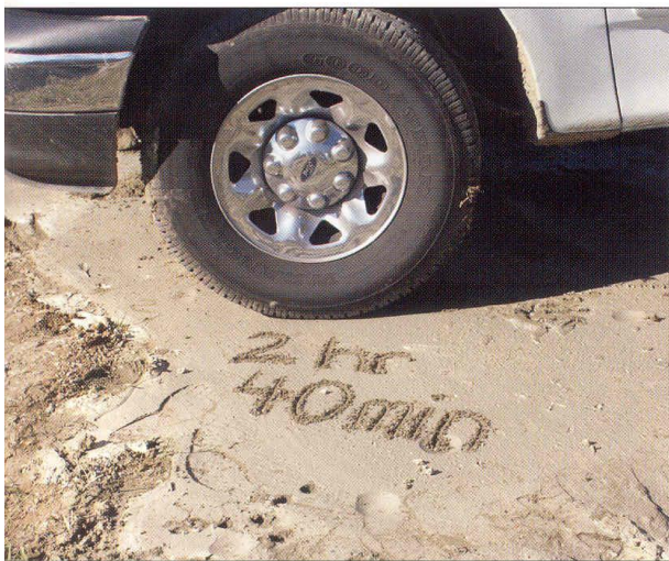
Figure 3. Full Size Club-cab Pickup on Early Strength Flowable Fill (ESFF) Trench at 2 hours 40 minutes
